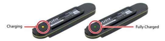
When connected to a power source, the charging LED on the back of the Hot-Swap Battery will illuminate. An amber light is displayed while the battery is charging and will turn green when fully charged. Charging may take up to two hours.
