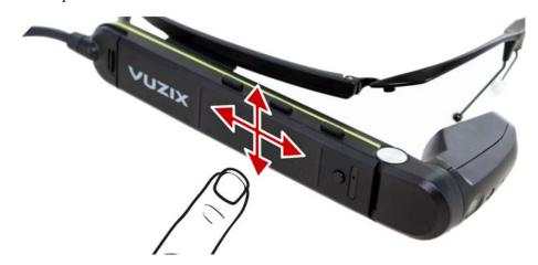
You can navigate through the M300 Smart Glasses interface by swiping up/down and forward/back. Double-tap the Swipe Pad to make selections.
